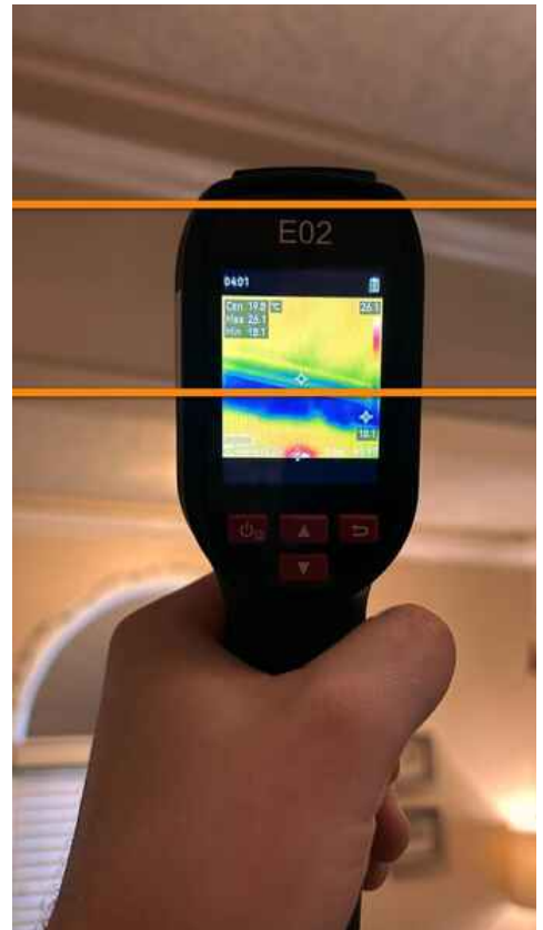
Cold spot is 18 while the rest of the room is 26
