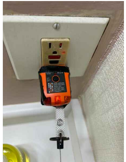
Outlet tester reads open ground
